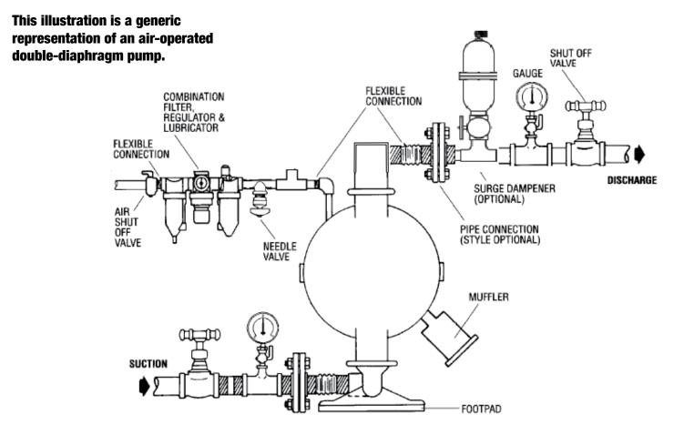
**NOTE:** In the event of a power failure, the shut off valve should be closed, if the restarting of the pump is not desirable once power is regained.
