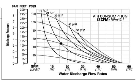
Flow rates indicated on chart were determined by pumping water. For optimum life and performance, pump should be specified so that daily operation parameters will fall in the center of the pump's performance curv
