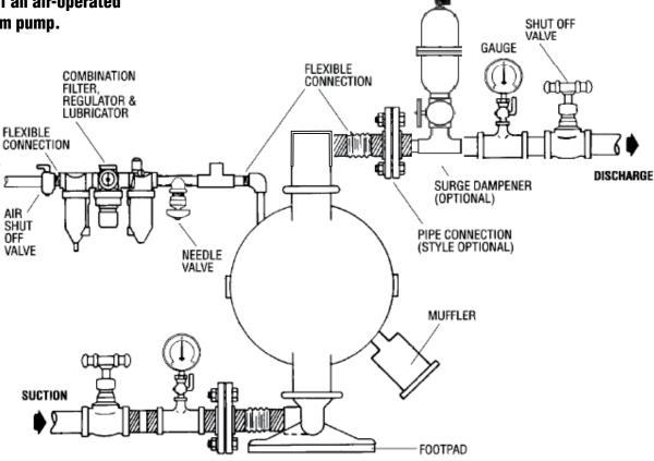
**NOTE:** In the event of a power failure, the shut off valve should be closed, if the restarting of the pump is not desirable once power is regained.
