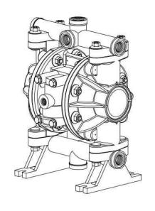
AIR-OPERATED O DOUBLE DIAPHRAGM PUMPS
